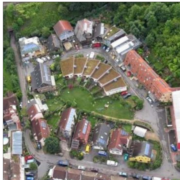
Ashley Vale, Bristol. Design principles were agreed, such as max. heights, roof pitch and a materials palette of timber, render and clay tiles to ensure a degree of continuity along the streets. Occupiers still had discretion regarding how to apply them to individual buildings. source: www.transitionbristol.net
